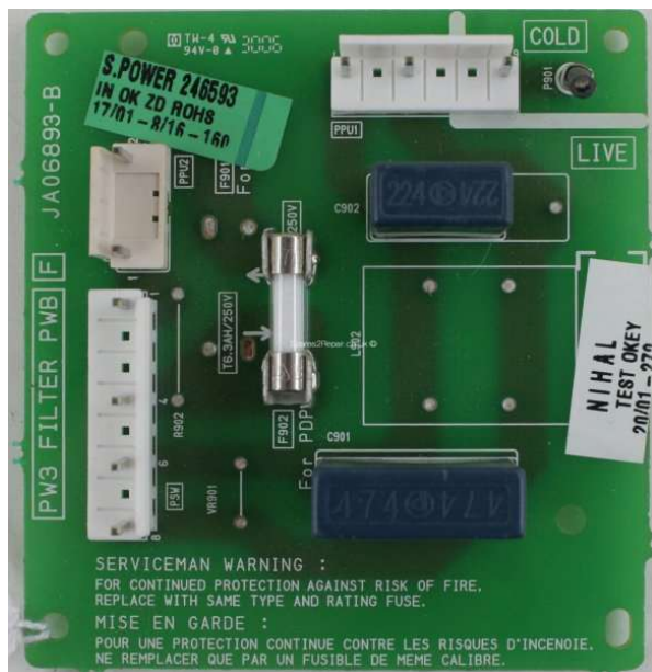
Figure 4.9 Example of fuse marking on PWB
