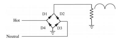
Rectification converts the sinusoidal AC line to DC with some ripple. When hot is positive with respect to neutral, current flows through diode D1, through the load (here a resistor), to ground, and then through diode D3 from ground back to the neutral. When it's negative, neutral is positive with respect to hot. Then the current flows through D2, through the load in the same direction, through D4, and then back to hot. Since current flows
