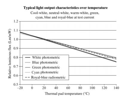
Constant current is the common way to drive LEDs, so this is a useful curve. But, in reality, it mixes two effects. With temperature, the efficacy decreases but the input power also decreases (because it comes with constant current). So, even though this curve shows the brightness decrease, it does not show the efficacy decrease.
